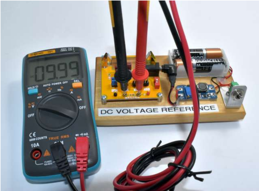
Fig 4 Use of the Voltage Reference to check the authors 6000 count DMM
