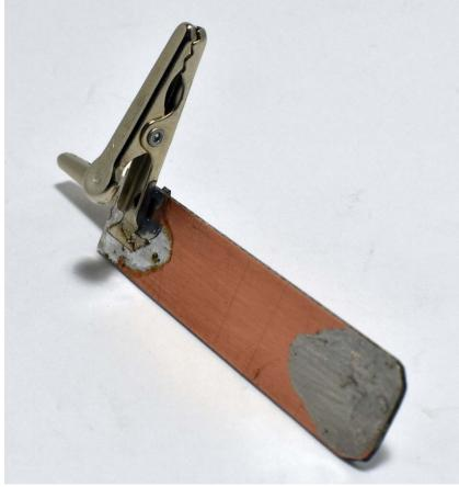
The photo to the left, shows the approximately 12 mm x 50mm strip of 0.78mm (0.031") double-sided copper pcb used for the adapter. Note for AAA batteries, the test end should be reduced to about 8mm wide.
