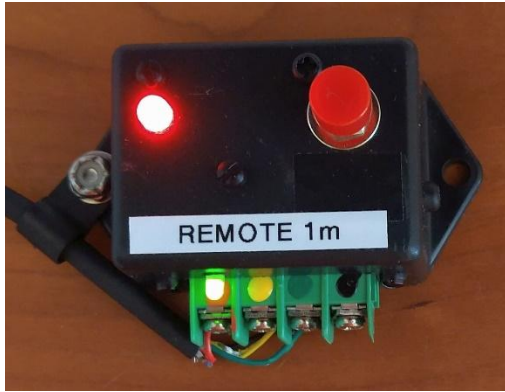
Fig 3 shows Remote #1 as an example which has been modified with the addition of the MPS, a home-made light-pipe and a new momentary pushbutton. On the topside you can see the illuminated light-pipe on the left. It is in contact with the led which is on the MPS bottom-side. The light-pipe is easy to make from 5mm acrylic rod or similar. See note 1 for guidance.
