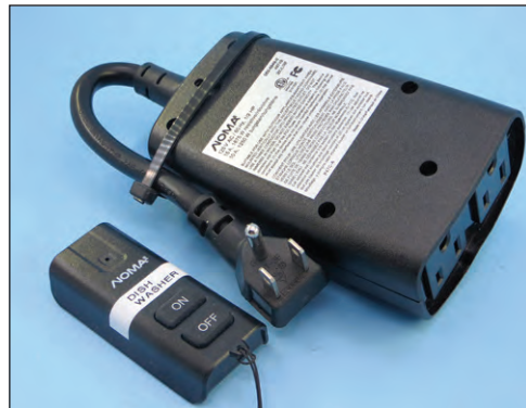
Figure 7: AC wireless switch with the remote on-off controller.
