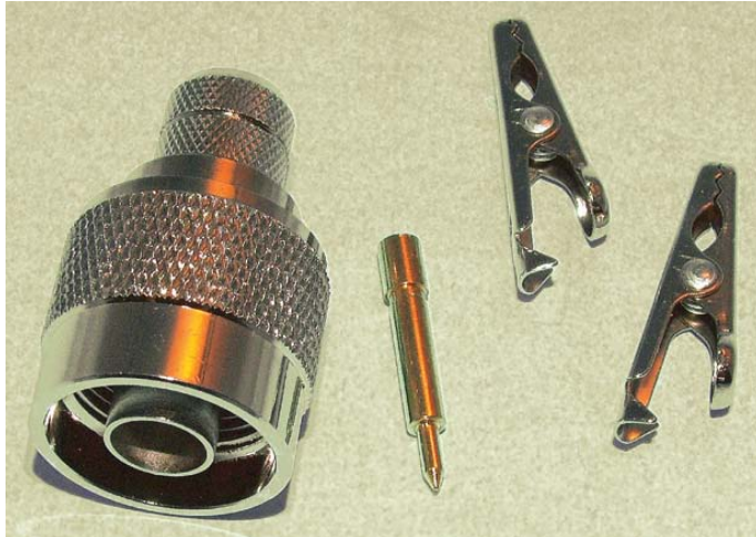
Figure 6 — The Type-N connector, its center pin, and the two alligator clips that make up the adapter. [Don Dorward, VA3DDN, photo]
