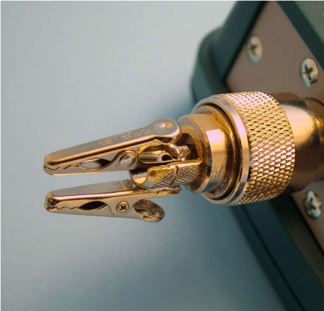
Figure 8----- This is version 2 of the adapter, with only half of the back end cut away. This design produced an improved SWR, [Don Dorward, VA3DDN, photo]
