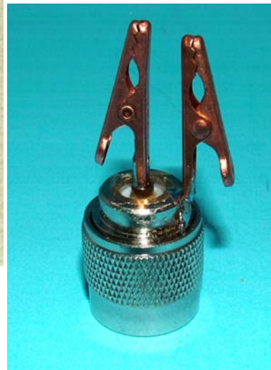
Figure 7 — Version 1 of the modified Type-N connector converted into an adapter for checking twinlead type lines. [Don Dorward, VA3DDN, photo]
