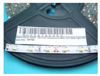
amber glow from the tiny lamps. Once again rooting in the junk box turned up a part reel of high brightness strip LED's, the kind that already have a current limiting resistor in series with 3 SMD LED's and operate from a nominal 12v DC. The led's come mounted on an adhesive backed copper strip and covered with a soft protective clear silicone coating to make them waterproof. They were intended to be cut off as required in multiples
