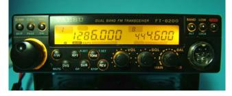
Photo 2 shows the new, improved backlit illumination on the FT-6200, using surface mount led's instead of the tiny lamps.
