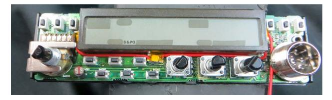
Referring to Photo 5, the radio front panel bezel has been removed and if you look closely, you can see the left (led1) and center (led2) led's ( the yellow dots!) mounted in place. Each led has had a small amber colored piece of tape stuck on to it. This was cut from a left over bit of 3m 5413 polyimide electrical tape. (Note, you could also use a piece of amber lens
