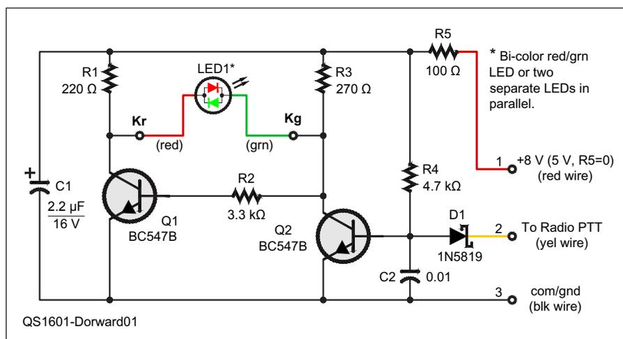
**Figure 1** — Schematic diagram for the microphone PTT indicator. LED1 is external to the printed circuit board and may be either a single bi-color red/green LED, or two separate cross-connected LEDs. Connect the cathode for the red LED to Kr, and the cathode for the green LED to Kg.
