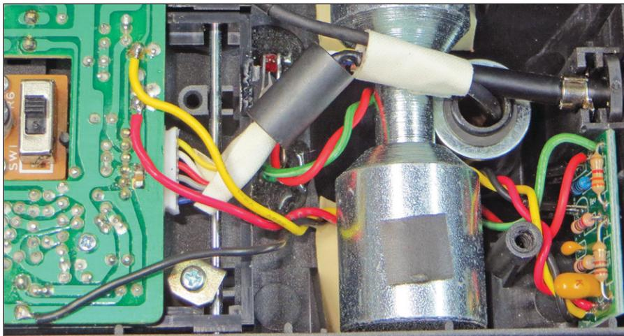
**Figure 3** — The PCB fits into the right side of the microphone base. Note the connections of the red, yellow, and black leads.
