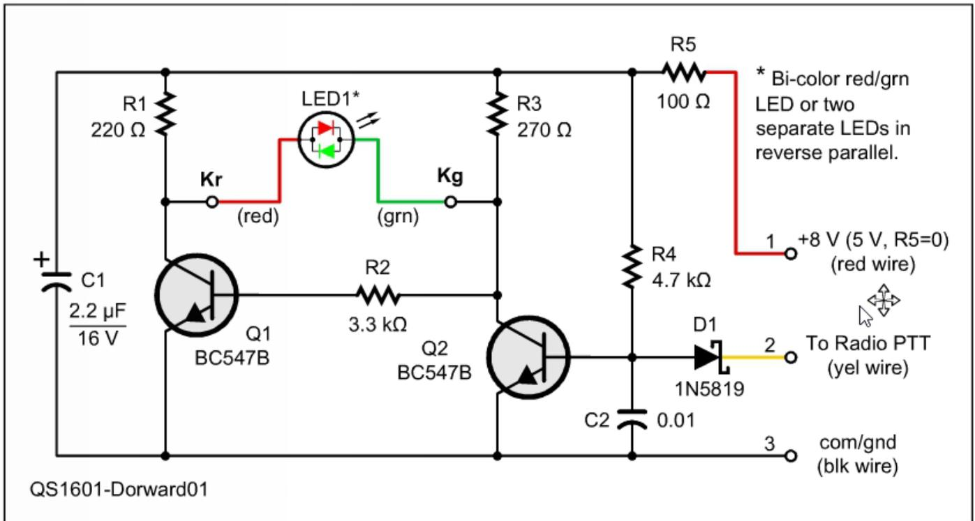
**Figure 1** — Schematic diagram for the microphone PTT indicator. LED1 is external to the printed circuit board and may be either a single bi-color red/green LED, or two separate cross-connected LEDs. Connect the cathode for the red LED to Kr, and the cathode for the green LED to Kg.
