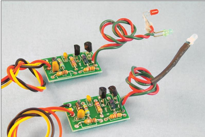
**Figure 2** — PCBs for a pair of colored LEDs (top) and a single bi-color LED (bottom) connect to the microphone by the red (+8 V), yellow (PTT), and black (ground) wires.
