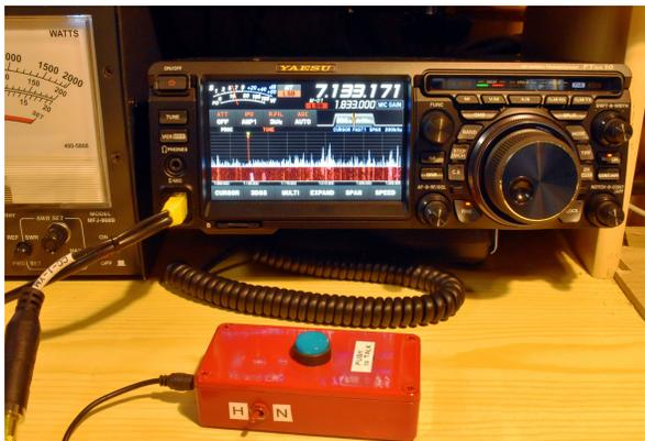
Fig 2 left shows the completed PTT switch in use. (using the NKK switch in the Hammond box, painted fire engine red!) (note: for a few
