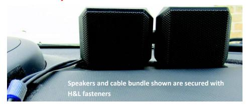
equipment securely mounted in the desired location. I have always found the strategic use of hook and loop fasteners to be a great help in this area. One big advantage is that there is no need to drill mounting holes or use screws or bolts. Another is the relatively easy removal of equipment when needed. However, there are some pitfalls to avoid and, since I have fallen into most, I will try to prevent you from doing the same.
