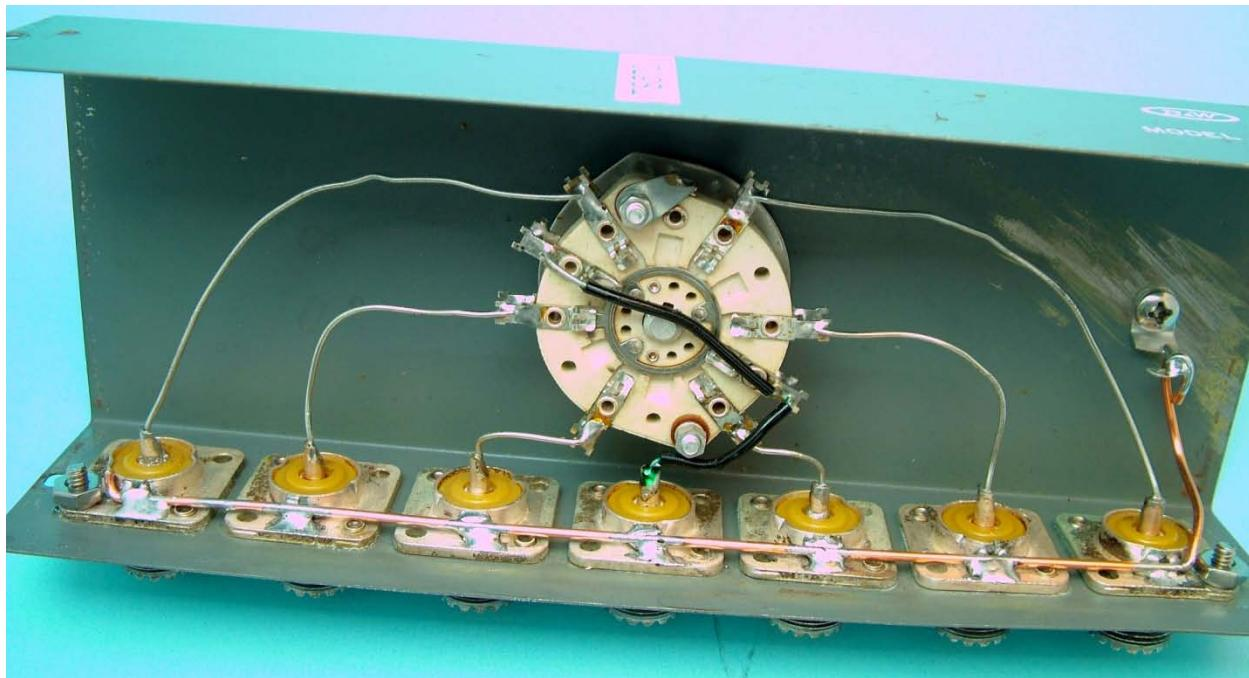
I drilled out 2 of the bulkhead connector rivets, one at each end of the connector "strip" and replaced the rivets with a stainless steel machine screw, lockwasher and nut, making sure to scrape away the paint in the area of screw contact.
