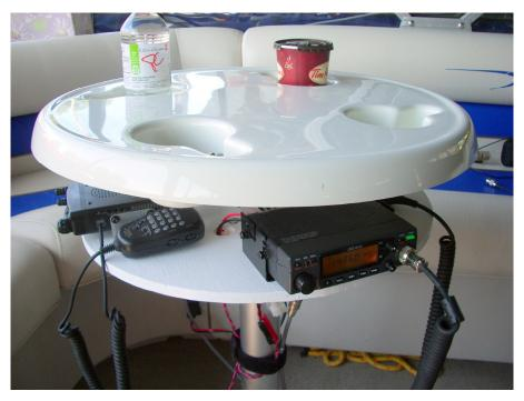
Many amateur radio operators are also avid boaters. No matter if it's a rowboat or even a large yacht, the issue of bringing along or mounting an amateur transceiver usually comes up sooner or later. In my case, I have a 21 ft pontoon boat and I was trying to decide how to mount 2 mobile transceivers in an out-ofthe-way, yet somewhat accessible location. I was looking at the floor-mounted pedestal table and it occurred to me that it would be neat to mount the radios
