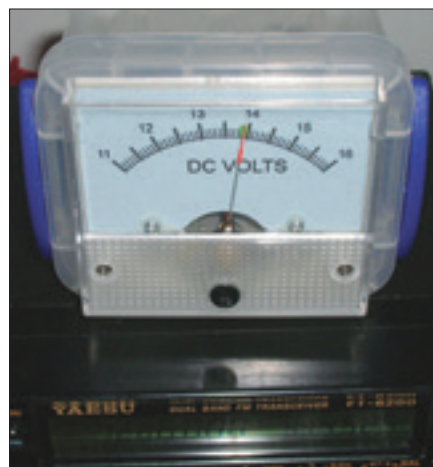
Figure 3 — This meter monitors the battery voltage in Don's, “kitchen shack.”
