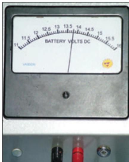
Figure 2 — A battery monitor meter with a customized scale added. The banana jacks on the front of the enclosure make it convenient to connect this monitor to any battery pack.
