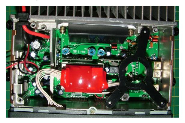
My ADI 247 became intermittent, with the RF output dropping off to zero after a minute of operation at full power. Eventually it would not operate on even medium power without the same thing happening.
